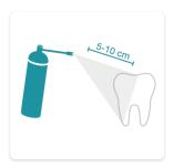
Apply SCANTIST 3D - vanishing from a distance of 5-10 cm. Spray the surface to be scanned.
